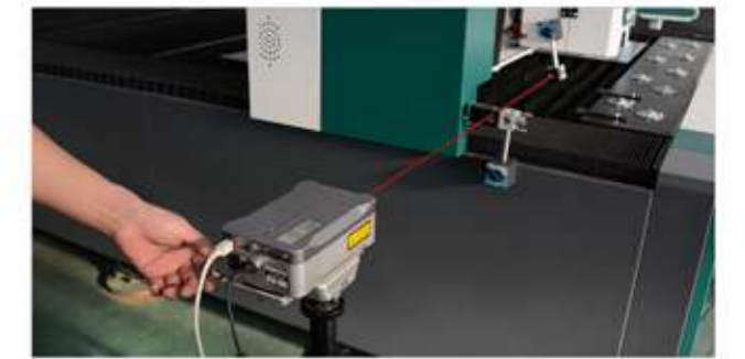
The laser interferometer guarantees the running accuracy of the whole machine
