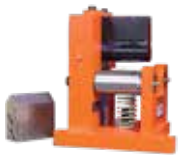
Weld Coupon Bender (L)
